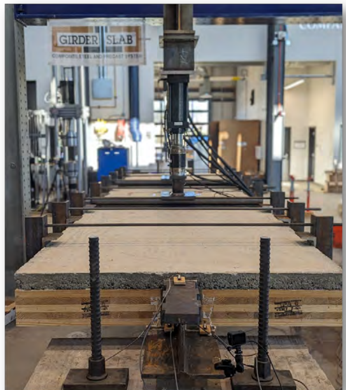
CLT TEST ASSEMBLY (AUBURN UNIVERSITY)
