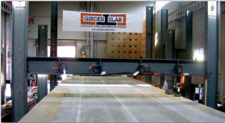
HOLLOW CORE TEST ASSEMBLY (VILLANOVA UNIVERSITY)
